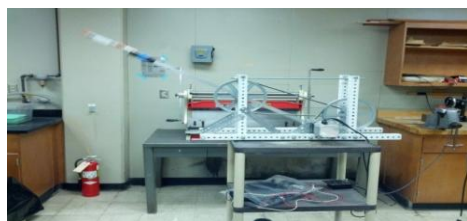
Figure 20: A sample rotating in the custom-made rotator
