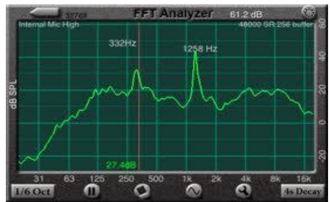
Figure 12: A sample Fourier analysis [47]. This sound wave has the most power at 332 Hz and 1258 Hz and has the least power at frequencies near 0 Hz.
