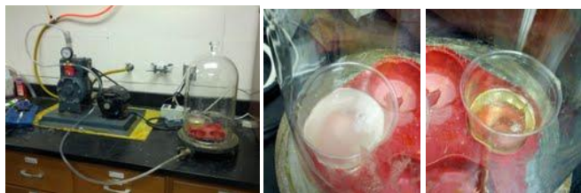
Figures 17, 18, and 19 (left to right): The bell jar evacuation chamber, bubbles forming in the epoxy resin, and bubbles forming in the epoxy hardener.
