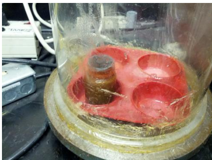
Figure 37: The unhardened 95% sample in the bell jar evacuation chamber.
